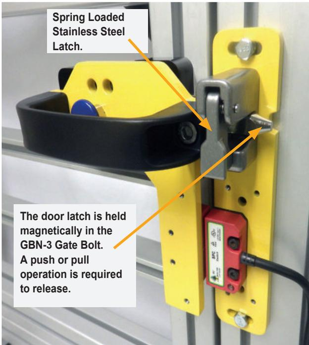
**GBN-3** shown fitted with SPF-RFID Non Contact Switch **Left Hand Version** shown.
