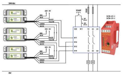
Three 2NC version switches connected in series to an SCR-21-i or SCR-31-i to give Dual Channel monitoring with Manual Start and Contactor Feedback Check
